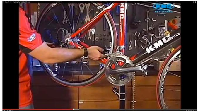
First thing we need to do is get the chain down to the smallest gear on the freewheel (rear) and the largest wheel on the chain wheel (front).
