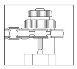
Step 2: Use Chain tool to pressure the pin in.
