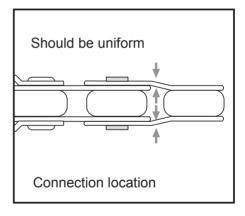
Step 4 : Be sure to check the connecting pin protrudes pin protrudes uniformly form both sides of chain the chain has been joined
