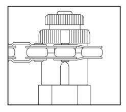
Step 3 : Make sure the pin is not over pushed. Pressure the pin in.
