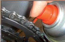
Lubricate into the chain's bearing
